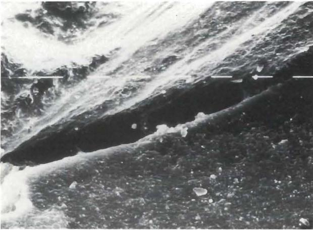
Figure 5. SEM photograph of a marginal gap which was not detected by direct and indirect assessment (640x).
