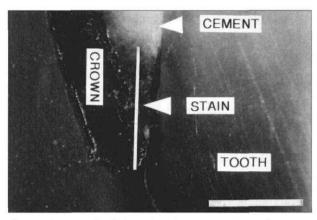
Fig 1. Micrograph of zinc phosphate cement specimen with some stain ingress. Wide horizontal scale line represents 500 µm. Narrow vertical line represents linear stain ingress measurement.
