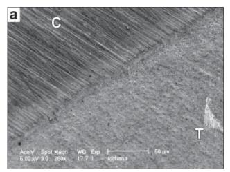
Figure 2A. Scanning electron microscope image of enamel specimens immersed in Powerade under 250X magnification, illustrating the erosive step between test and control areas of enamel. Image taken at boundary of test (T) and control (C) areas.
