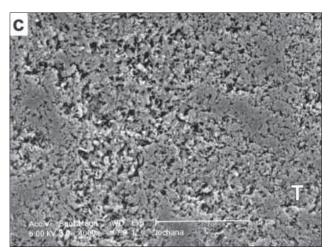
Figure 2C. Specimen in Powerade under 4,000X magnification, illustrating the irregular etch pattern.
