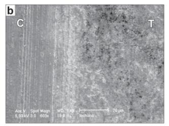
Figure 3B. Specimen in Powerade plus 0.125% casein phosphopeptide-amorphous calcium phosphate under 600X magnification, illustrating discrete areas of surface irregularities.
