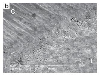
Figure 2B. Specimen in Powerade under 1,000X magnification, illustrating step between test and control areas of enamel.
