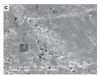
Figure 3C. Specimens in Powerade plus 0.125% casein phosphopeptide-amorphous calcium phosphate under 4,000X magnification, illustrating surface globules over enamel test areas.
