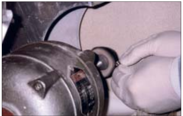
Figure 9. Final finishing and polishing completed on lathe with Tripoli and jeweler's rouge on cloth wheels.
