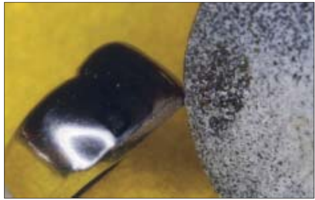
Figure 7. Rotating counterclockwise in this view, the heatless stone thins the margin and applies a "minicrimp" to crown edges.
