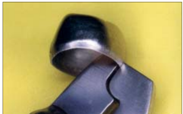
Figure 6. The crimping pliers bends edges inwardly.
