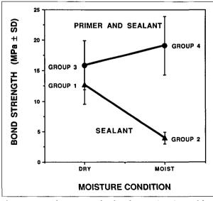
Figure. Mean shear strength of sealant and sealant with primer under dry and moist conditions.
